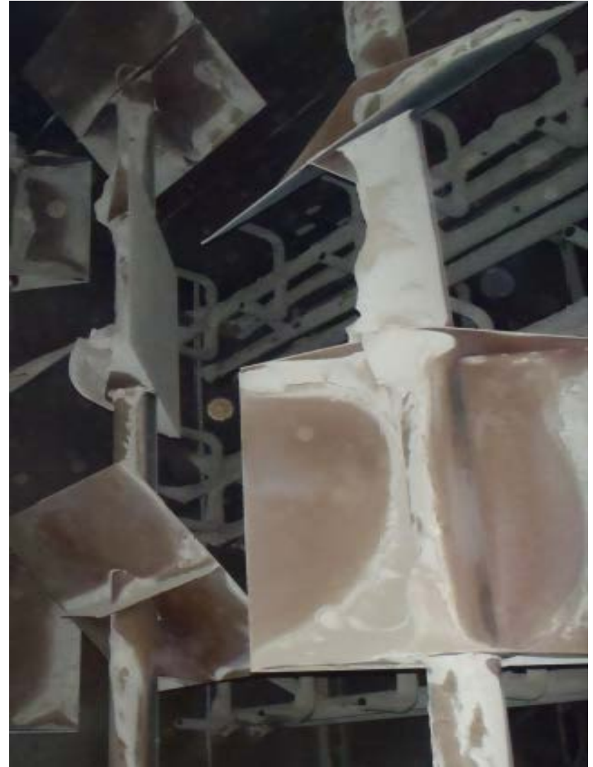
LPA Screen damaged by falling ash clumps
